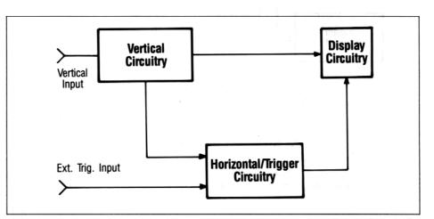
Fig. 11. Simplified oscilloscope block diagram.
