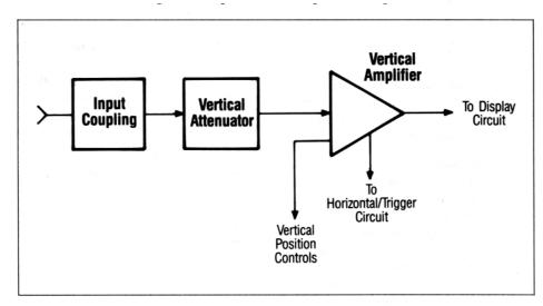
Fig. 12. Vertical circuitry block diagram.
