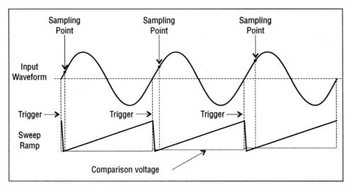
Fig. 19. Equivalent time sampling.
