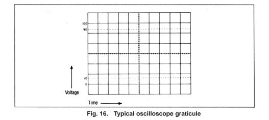
is marked with two dashed lines, labeled "10" and "90" and points marked "0" and "100" are also present. These four points are useful for rise time and fall time measurements, since rise time is defined as the time required for a signal to rise from 10% to 90% of its maximum amplitude. On almost all modern oscilloscopes, the graticule is etched directly onto the inside of the CRT. This eliminates parallax error that might occur from viewing the CRT from a slight angle.
