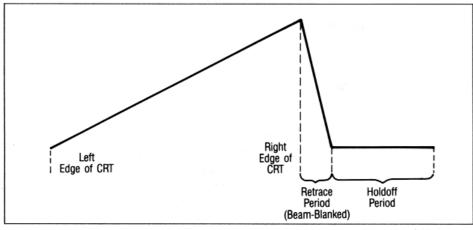
Fig. 15. Sweep waveform.
