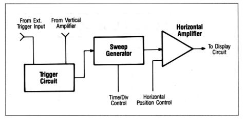
Fig. 13. Horizontal/trigger circuitry block diagram.
