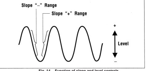
Fig. 14. Function of slope and level controls.
